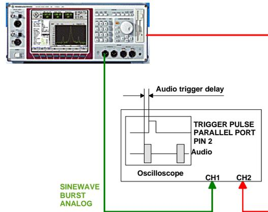
Fig 2 R&S UPL time offset between trigger pulse and sine burst without compensation.
