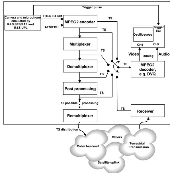
Fig 5 The audio-to-video delay measurement scenario.
